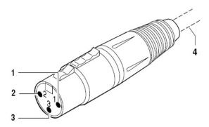
1 dc supply (+) 3 Chassis ground 2 dc return (-) 4 Cable wires
